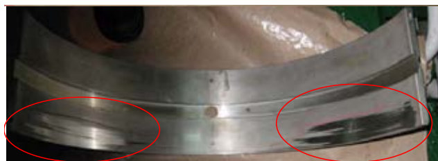
Upper main bearing shell
