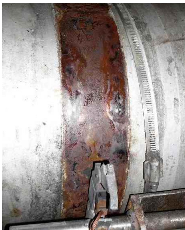
Corrosion hiding behind the slip ring
