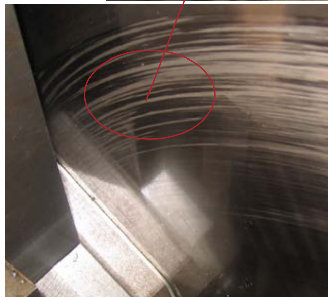
The greyish stripes on this thrust collar face indicate spark erosion
