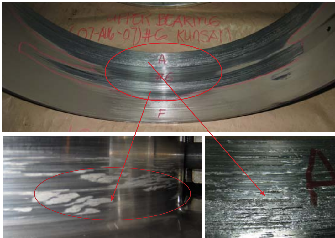
Upper main bearing shell
