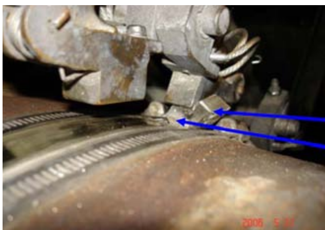
Poorly adjusted brushes
