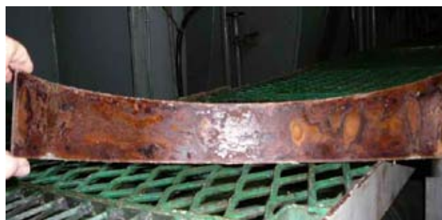
Heavy corrosion on the back side of the slip ring
